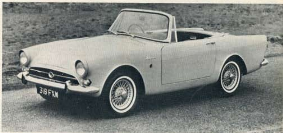
The Series II Alpine, fitted with a 1592cc engine. Many of the mechanical components are the same as the SIII Rapier.
