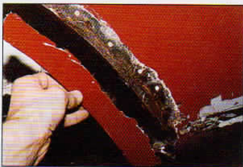
Glassfibre wheelarches were cut away and replaced
