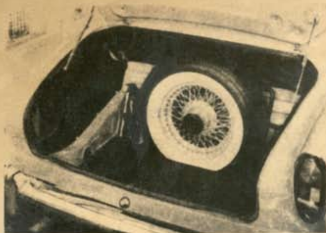
Now that the fuel tanks have been put inside the fins and the spare wheel mounted vertically, luggage space is really useful.
