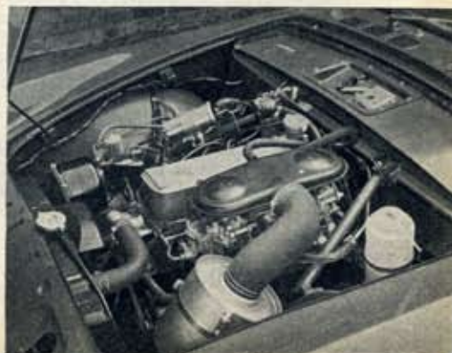
A new air cleaner-silencer and revised exhaust manifold with a single down pipe are calculated to make the G.T. model considerably quieter than the Sports Tourer
